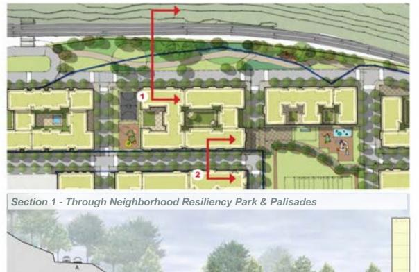
The Street Sections diagram illustrates the proposed right-of-way widths around the Main Campus, and the conceptual building setbacks. The right-of-way is the area controlled by the City typically consisting of the travel lane, bicycle lane, curbside zone (parking, loading, etc.), furnishing zone (street trees, light poles, benches, etc.), the sidewalk through zone, and the frontage zone. The Hoboken Complete Streets Design Guide provides a visual representation of these elements:
